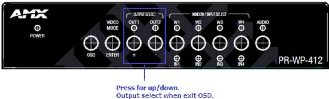
Press to select input or press to select the current window layout display when on Multiview mode.
