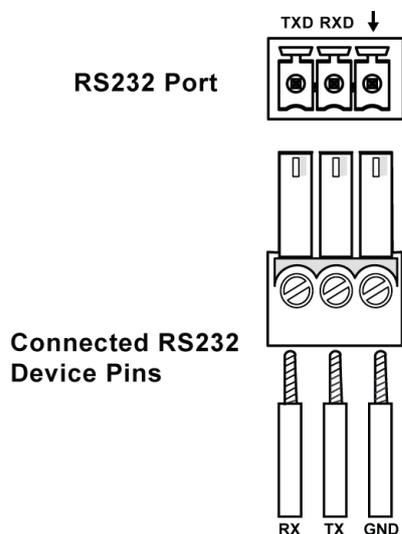
RS232 port is used to control the processor through RS232 serial communication.
