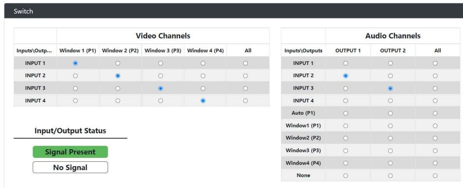
The input/output switch allows selection of output port (display) and input port (source) for specific combinations of displays and sources within the matrix.
